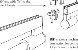
STJR-creates a mechanical connection for continuous runs. One connector is included with each two connecting fixtures.
